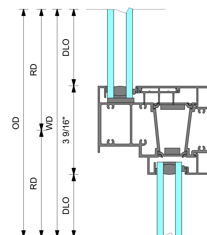
3 DETAIL 3 OS FIXED OVER PI REPLICA MEETING RAIL ASSEMBLY NON-BEVEL FACE
